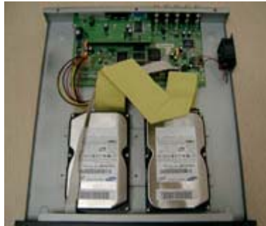
Two HDD Installation
