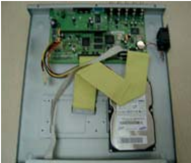
One HDD Installation
